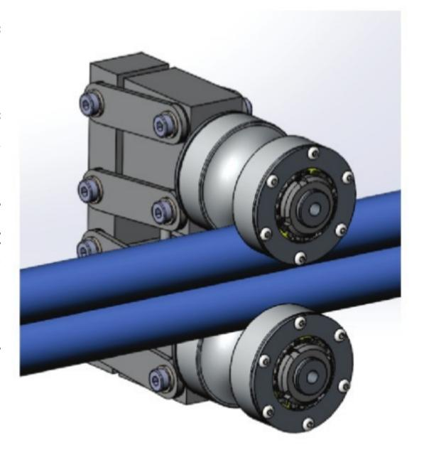
With this innovative technology, another notable advantage comes into play which is called the "snake effect". The ropes will distribute the stretching angle applied equally between all guide elements
